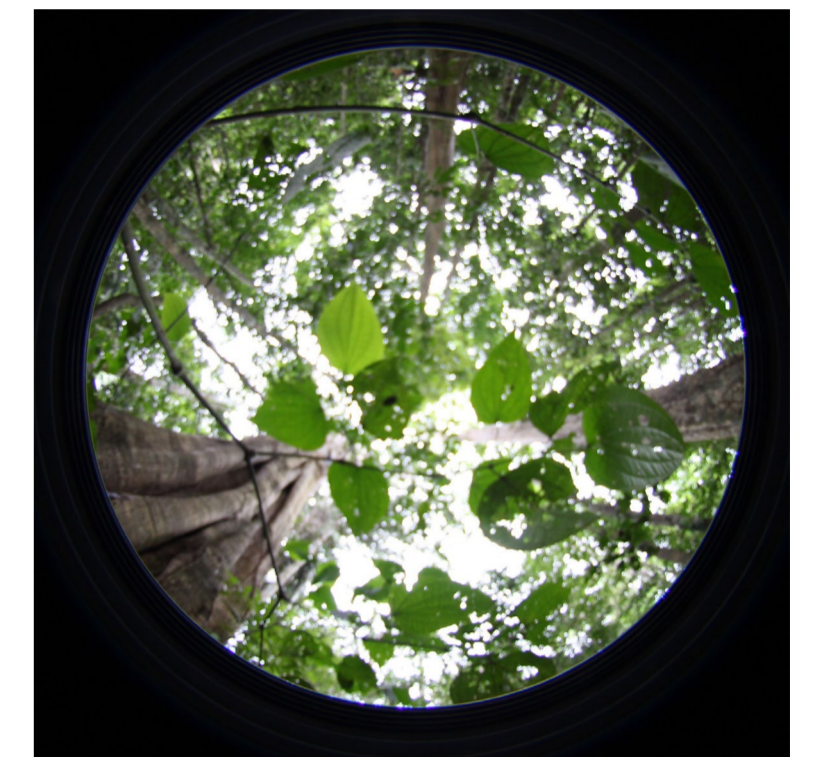
Figure 4. Canopy images are taken at 3 exposures and analysed to calculate canopy density.
